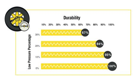
Tyre durability according to pressure loss percentage.
